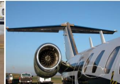
Figure 4(b).—Horizontal and vertical tail ice for the wing ice protection system failure case.
