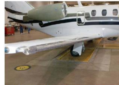
Figure 4(a).—Wing ice protection system failure case.
