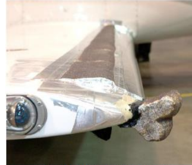
Figure 3(a).—Upper wing runback shape.
