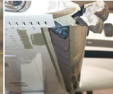
Figure 3(b).—Lower wing runback shape.
