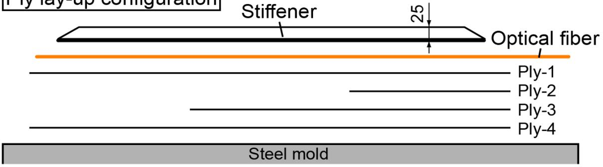
Resin saturating preforms bonded stiffeners and skin
