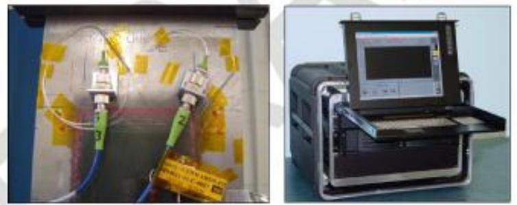
FIGURE 20 - FIBER OPTIC SENSORS IN ADHESIVE BONDLINE AND FO MONITORING EQUIPMENT
