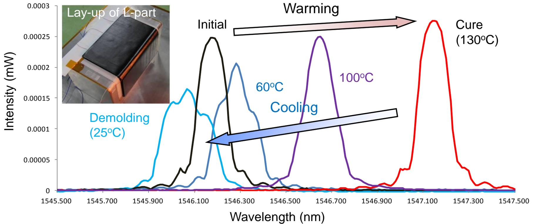
Spectral shape changed during cooling and demolding process due to cross-sectional deformation of optical fiber (birefringence effect)
